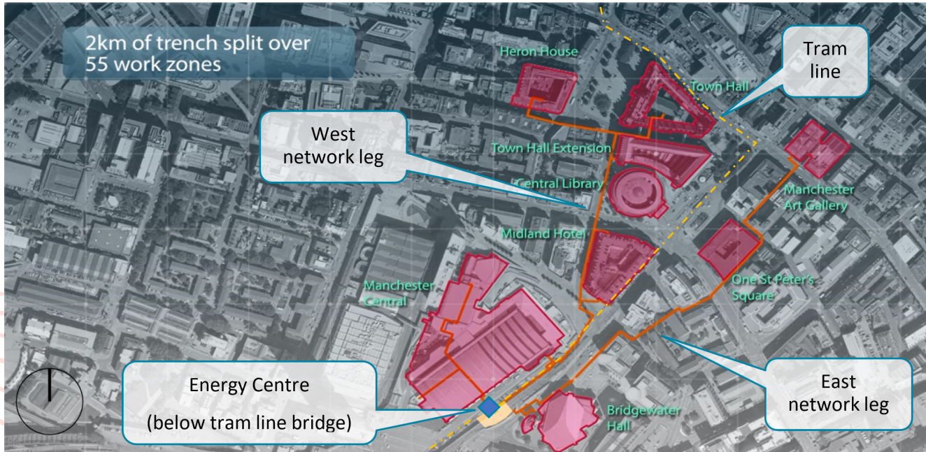
Figure 1. Location of Manchester Civic Quarter Heat & Power Network and Energy Centre – note Midland Hotel will no longer connect to the network. (adapted from Vital Energi drawing)
